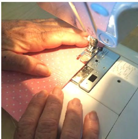
2. Regular sewing machine: Stitch 1/4" from the folded edge to secure the fabric / interfacing. This is where the wire will be inserted & centered later.
