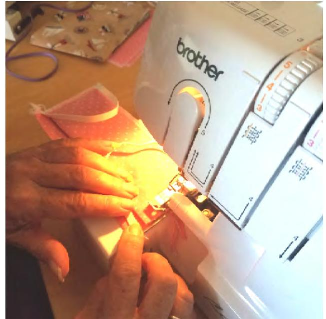
13. When you attach the bottom of the elastic, make sure the elastic is not twisted & will lie as flat as possible when placed on a face. Attach elastic to other side of mask in the same manner.
